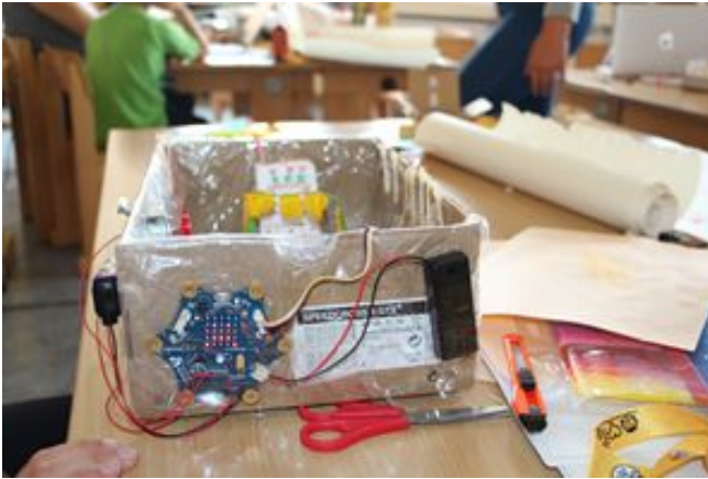
Figure 5: Cellar moisture alarm
