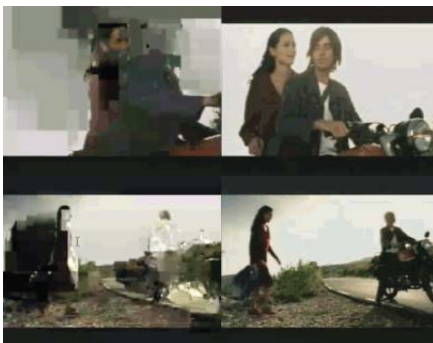
Real Player application in overloaded situation Left: standard service, right: premium service with 256 kbit/s bandwidth reservation
